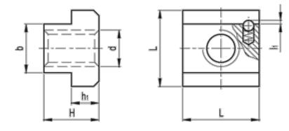
b -0.1 -0.3 = 14 d = M12 H = 16 h1 = 8 L = 22 I1 = 1.0 T-slot width DIN 650 = 14 Weight (g) = 34
